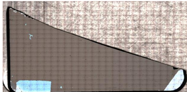
Fig. 2. Fragment 60000 color-enhanced to show increased blueness of silicon areas near focal point, presumably due to irradiation. The bright areas are silicon, called “heel” and “toe” of sock shape.
